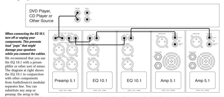
same. Also, XLR/balanced connections follow the same paths as the RCA/unbalanced connections described below. Since most audio systems are configured in stereo, this diagram includes two EQ 10.1s. You may use either of the two for the left or right channel. If you have a single EQ 10.1 in a mono setup, simply adapt the diagram above by omitting one of the stereo connections.
